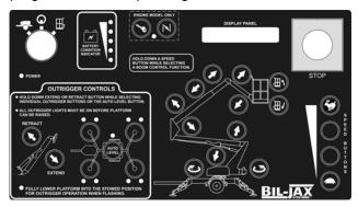
Figure 2-2. Boom Lift Control Panel (Ground)
